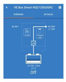
The button the on left will allow you to limit how much amperage you can draw from your shore power source. By default, it will be set to 30A as the trailer uses a 30A inlet plug. However, you may want to change this limit temporarily if you are on a 20A or 15A outlet to prevent tripping the breaker on your power source.
