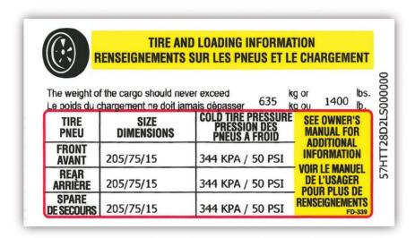
The Cargo Carrying Capacity label provides cargo loading information and is located on the jamb of the entry door. *Example*:
